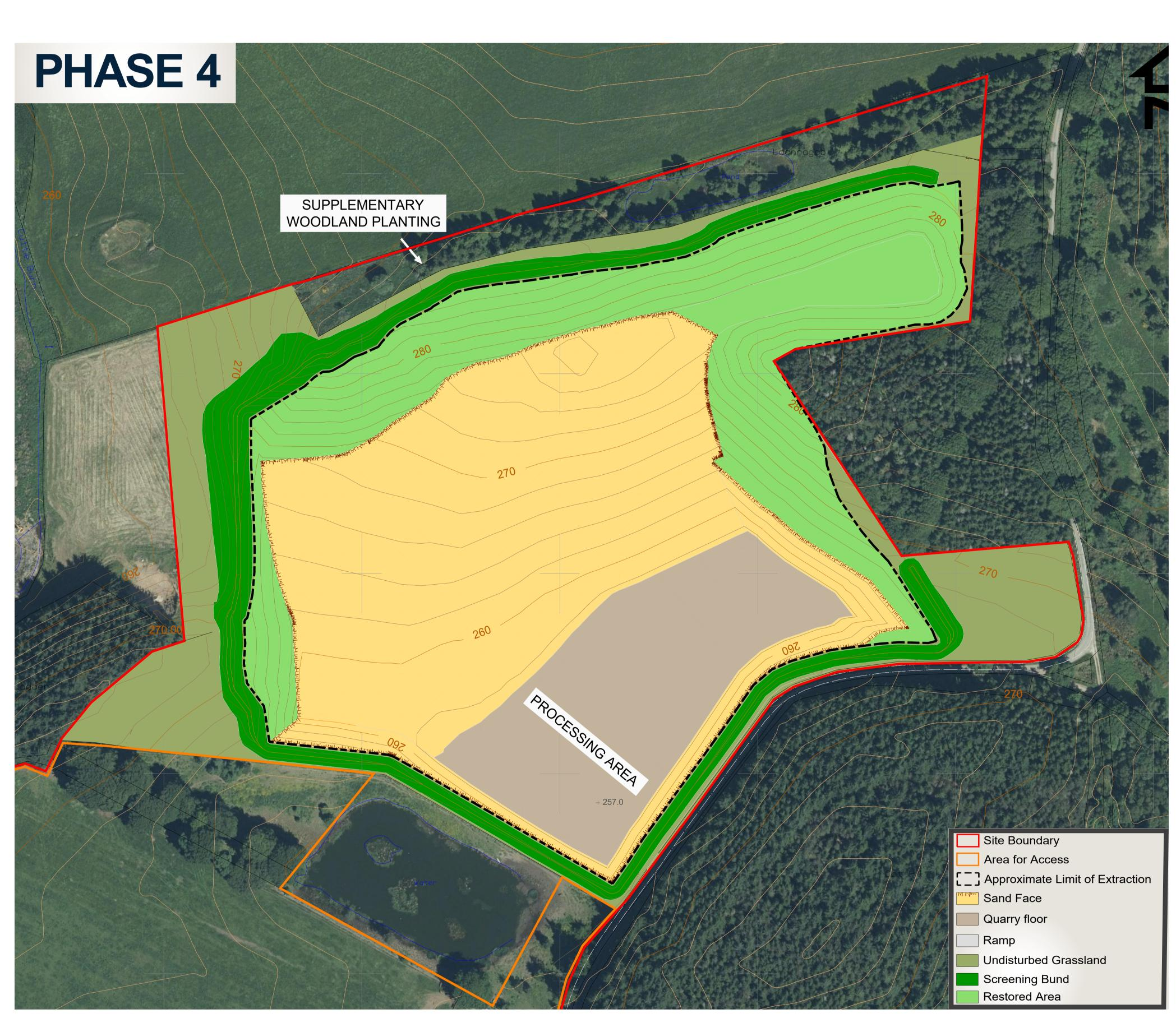
In Phase 4 the quarry floor will be worked to its maximum Southern extent with the excavation deepened to 257m AOD across a wider area. Progressive restoration would be undertaken on the Eastern and Western boundaries of the excavation area using soils stripped from the Phase 4 area and directly placed. It is anticipated that operations in this phase will take approximately 5 years.
