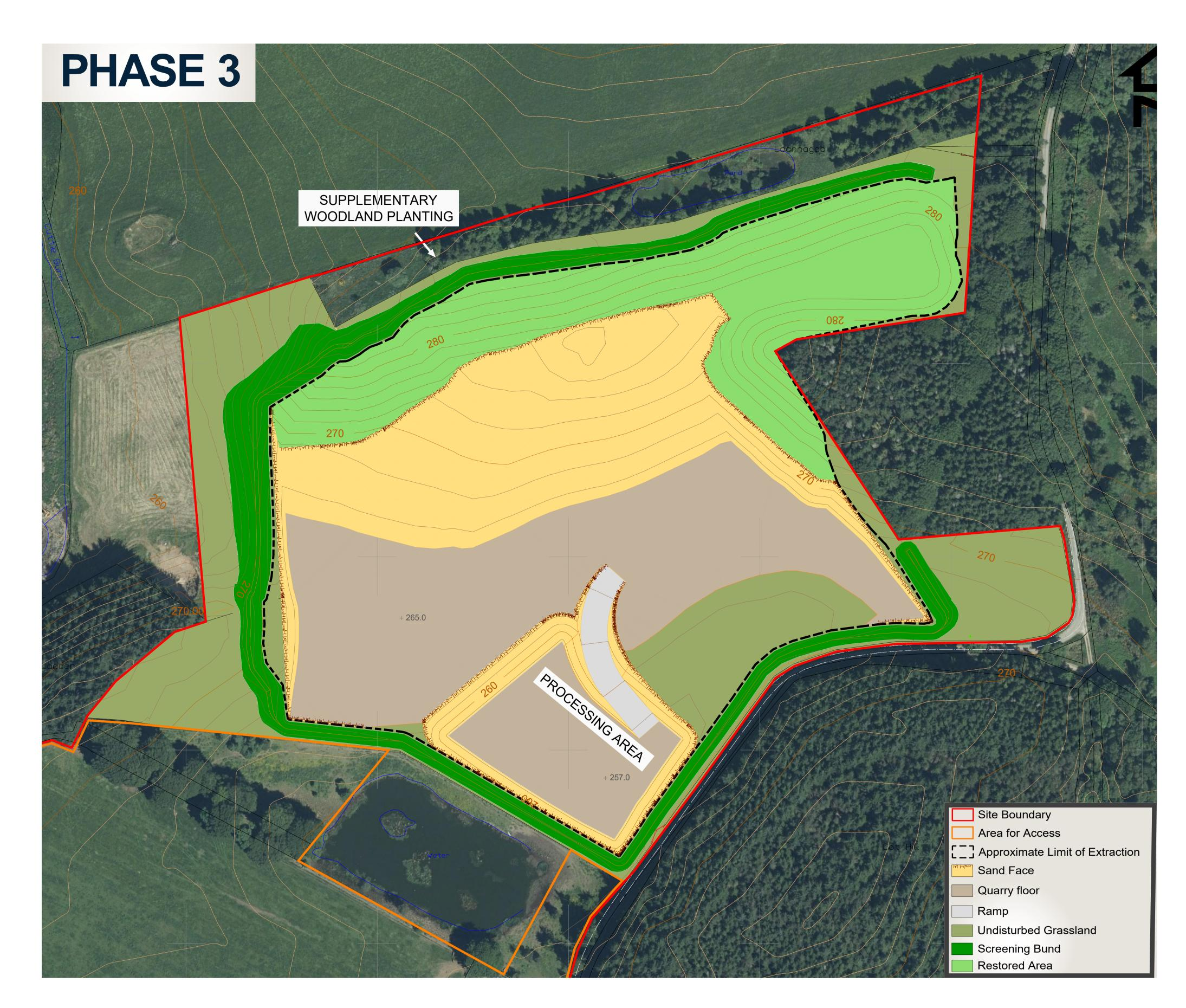
In Phase 3 the quarry floor is extended in a Southerly direction and deepened to 265m AOD. Progressive restoration will continue in this phase, with the remaining Northern quarry faces reprofiled, soiled and seeded/planted using soils stripped from the Phase 3 area and directly placed. It is anticipated that operations in this phase will take approximately 6 years.
