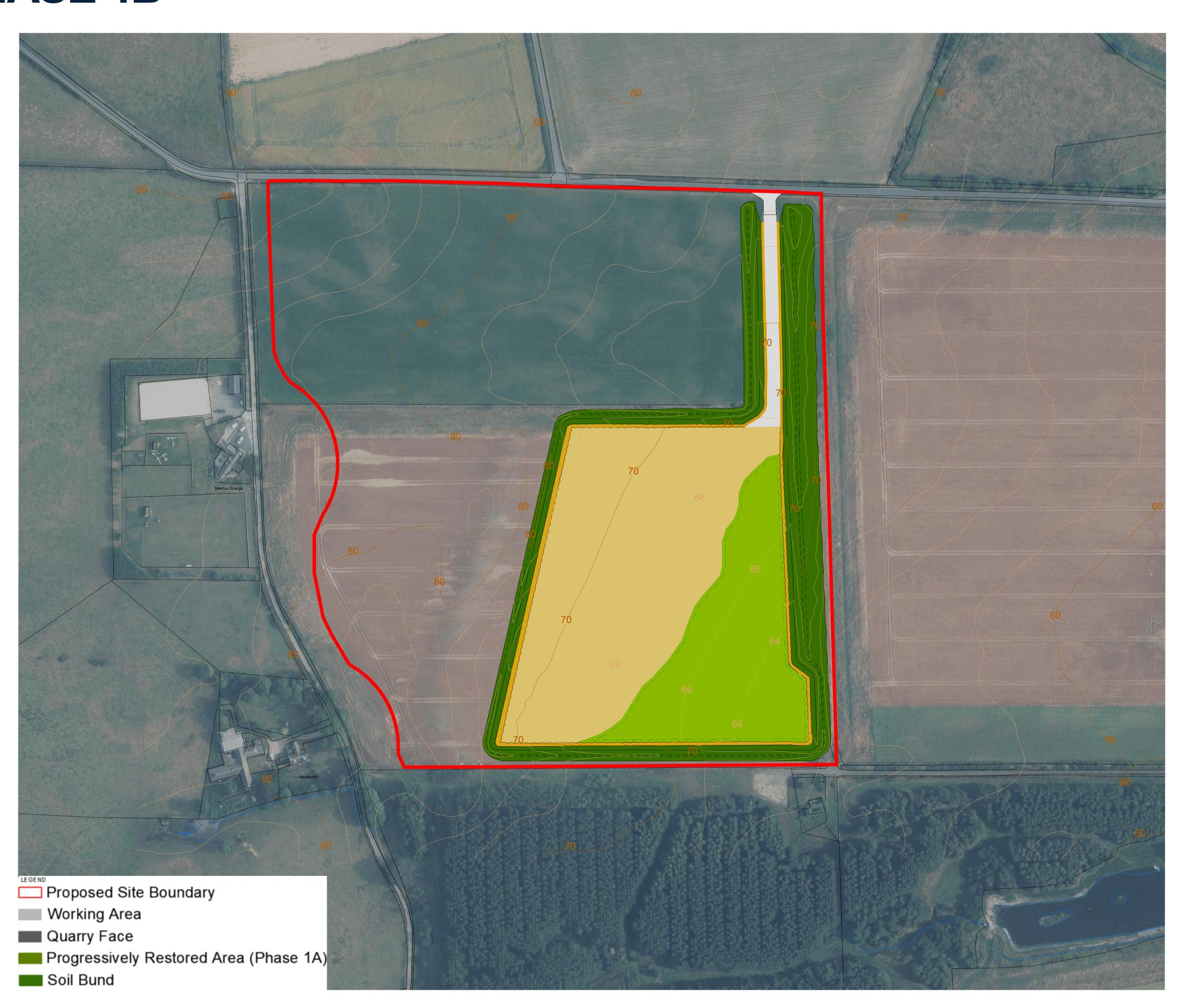
In Phase 1B the excavation would be extended westwards within the southern field. Soils and overburden stripped in Phase 1B would be placed and seeded to create a screening bund around the working area and used in progressive restoration of the Phase 1A extraction area. Mineral extraction in this phase would take place over 1.5 years.
