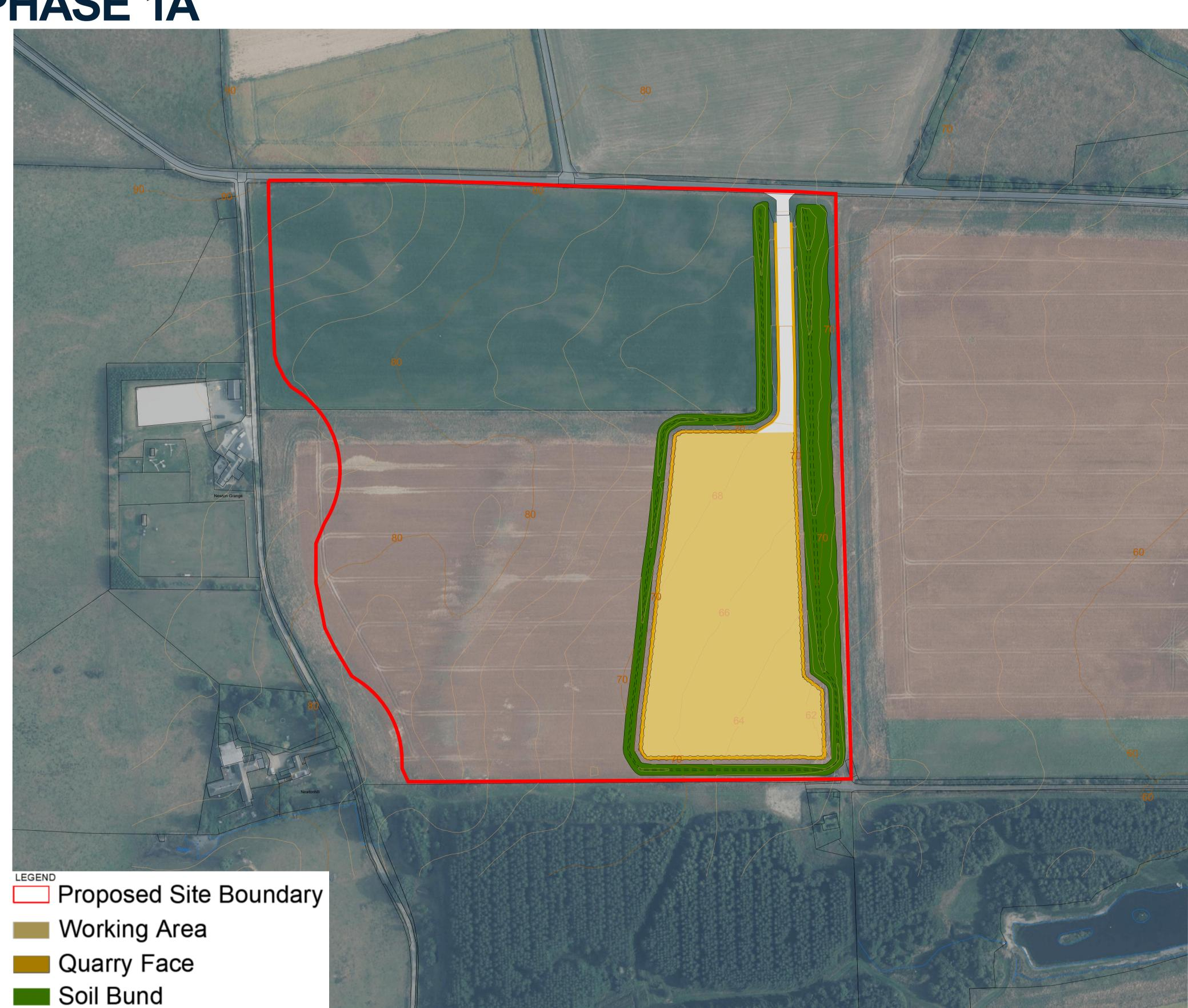
Initial excavation would take place in the south east of the site. Prior to extraction, soils and overburden would be stripped and placed in screening bunds around the periphery of the working area.
